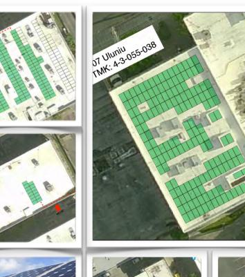
PRODUCTION 13,219 kWh / mo 158,626 kWh / yr 3,736,578 kWh / 25yr
